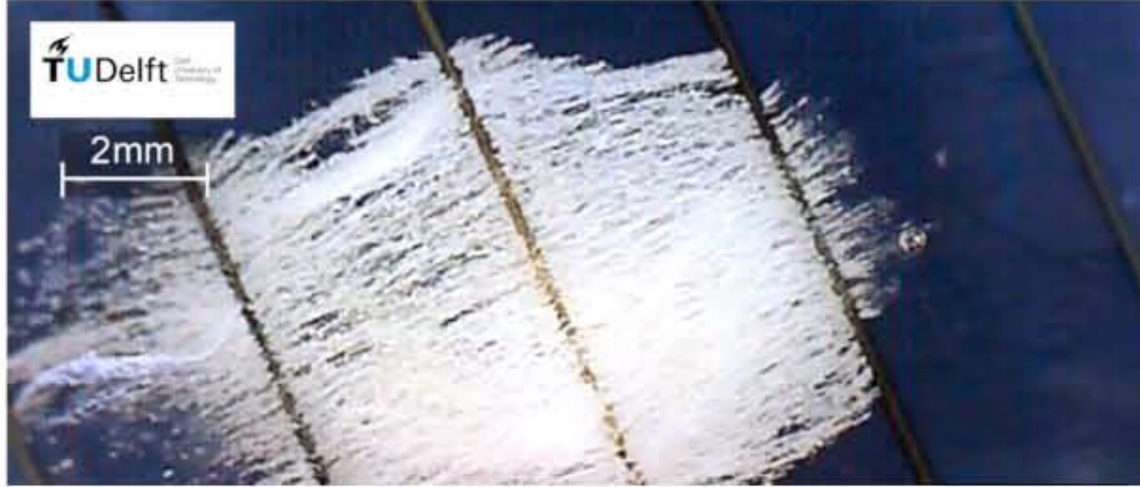
Dielectrophoresis of KNLN particles in UDMA, at 1kHz and 1kV/mm
